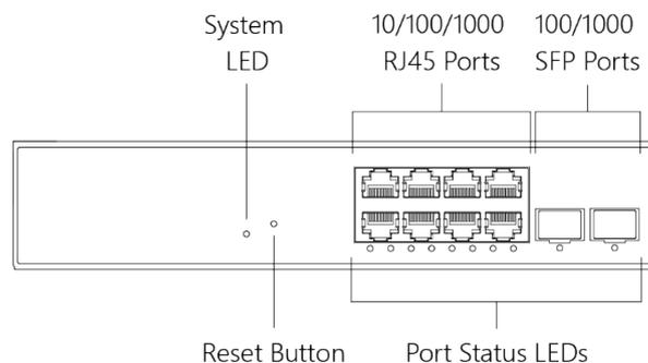
**Figure 1: Front panel of the switch**
