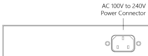
**Figure 2: Rear panel of the switch**
