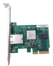
Megabit Ethernet (100MbE) over Cat5e/Cat6 or better cabling. This Multi-Gigabit NIC designed for low-power, low profile PCIe small form factor and single-port solution enabling pervasive NBASE-T connectivity.
