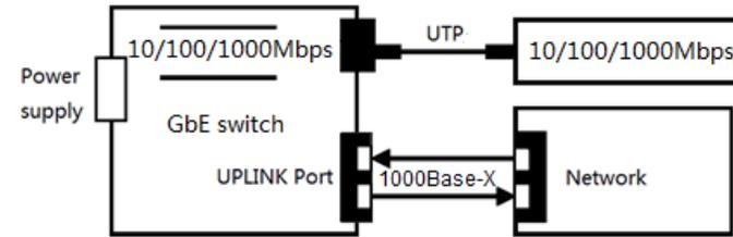
Connect one end of the standard UTP CAT5 network cable to the 10/100/1000Mbps RJ-45 ports on the front panel of the switch. Connect the other of the cable to the typical network devices.
