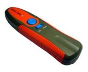
The universal connector can be used for all the most widespread fiber interfaces such as ST / SC / FC connector. It is suitable to test both Singlemode and Multimode cables. With an optional 2.5 mm to 1.25 mm optional Adapter, you can easily test 1.25 mm diameter fiber LC connector. The visibility is up to 3 Km to 5 km depends upon the output power of the Fiber Checker.
