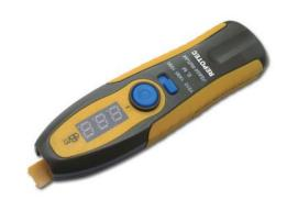
equipments or other optic sources. It measures power in both 850 nm / 1300 nm (Multi-mode) and 1310 nm / 1490 nm / 1550 nm (Single-mode) respectively.
